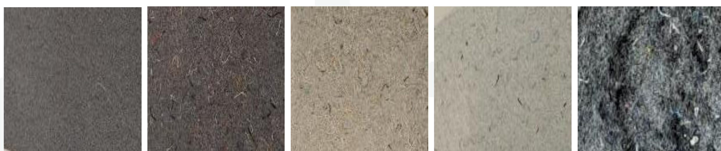
Figure 2. Lyocell-containing feedstock at different pretreatment stages and reject polyester fibres filtrated from the lyocell feedstock after the final stage of bleaching. From left to right mechanically refined lyocell, acid-treated lyocell, dithionite-treated lyocell, peroxide-treated lyocell, and polyester fibre reject from the lyocell-containing feedstock.
