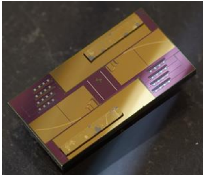
Figure 5 Two SLEDs mounted on a MIREGAS silicon photonics chip.
