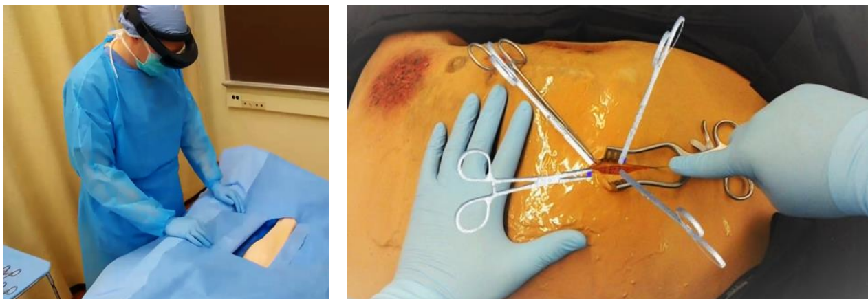
Figure 2. Left: Our AR HMD-based telementoring system being worn by the mentee. Right: First-person view of mentor-authored annotations (virtual instruments) anchored to the operating field.
