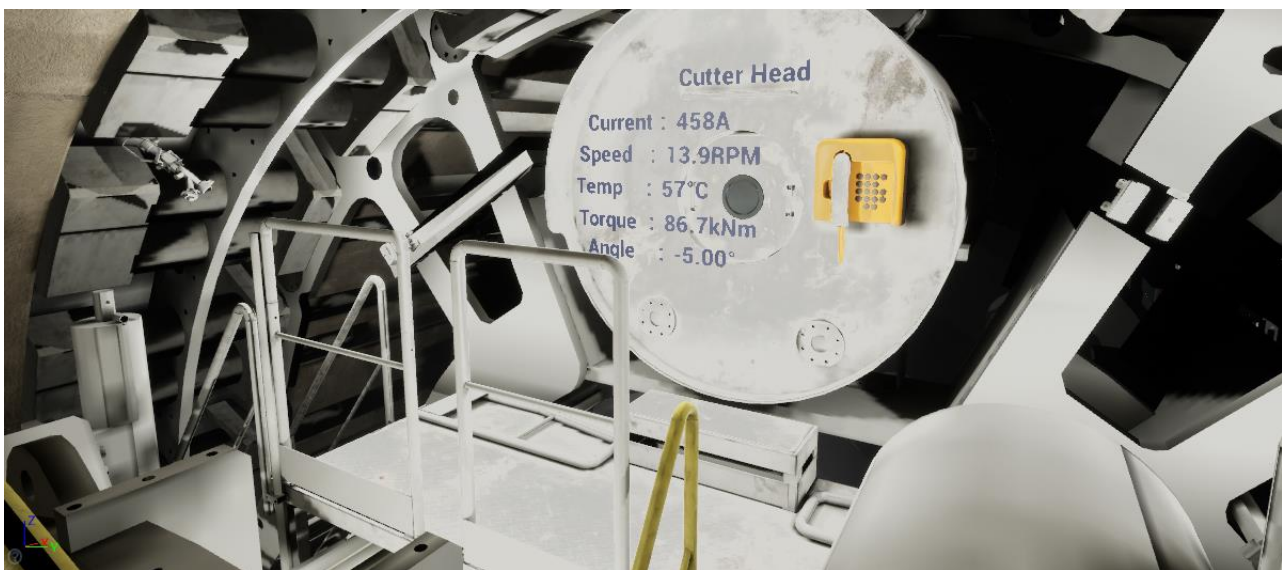
Figure 4. Display feed for the cutter head showing key overall values for the complete head.
