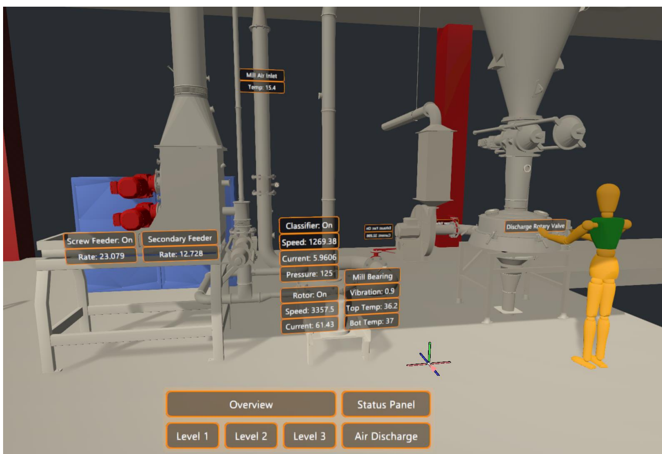
Figure 2. Hosokawa Micron Ltd. monitoring digital twin of a air classifier mill.
