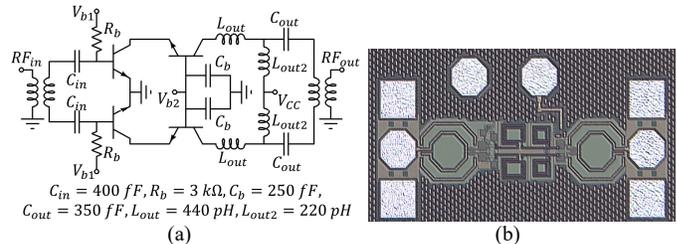
Fig. 1. (a) Simplified schematic of the LNA. The bias network is not shown for simplicity. (b) Micrograph of the LNA. The chip size is 620  $\mu\text{m}$  x 325  $\mu\text{m}$  including pads.
