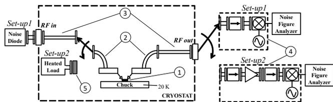
Fig. 2. Diagrams of two noise figure set-ups: *Set-up1* uses a noise diode and *Set-up2* uses a heated load, as noise sources. (1) Device under test, (2) WR-15 probes, (3) WR-15 waveguide set, (4) down-conversion block and (5) WR-15 thermal insulator.
