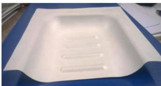
Figure 1. A sample of a tray with requirement of high extensibility.
