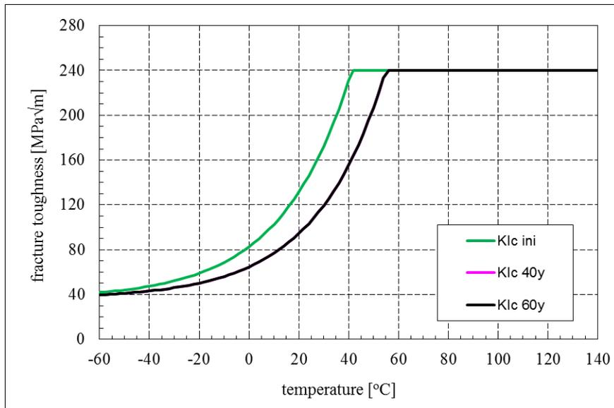
**Figure 3-4.** The resulting  $K_{Ic}$  transition curves after 0, 40 and 60 years in operation. In the legend “ini” is at the start of operation, “40y” is after 40 years of operation, and “60y” is after 60 years of operation.
