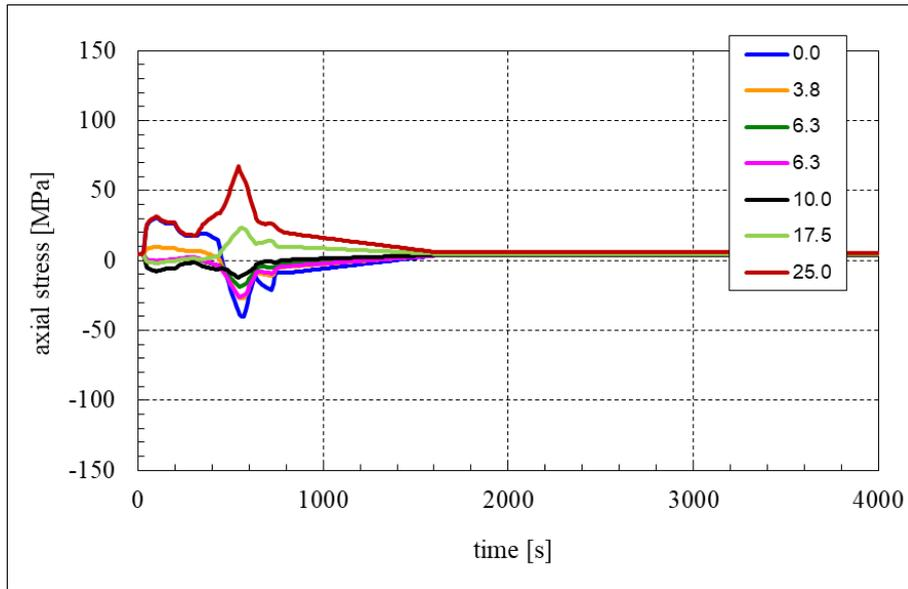
**Figure 4-3.** ADS transient => Core shroud wall axial stress time history (0 is at inner surface).
