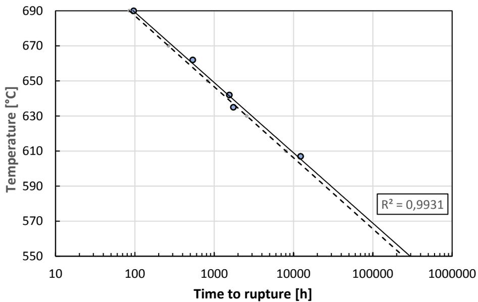
**Figure 2.** Isostress (69 MPa) cross-weld rupture test results of an ex-service P91 pipe (points with MH fit, solid line) in comparison to the upper range of P22 parent material scatter band (ISO data, dashed line)
