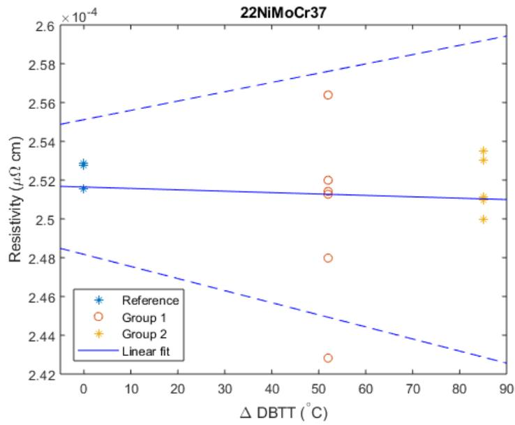
**Figure 3.** Resistivity and  $\Delta$ DBTT. For 22NiMoCr37 no correlation between resistivity and  $\Delta$ DBTT can be seen. However, the  $\Delta$ DBTT for the highest level of irradiation is significantly smaller than for other materials studied.
