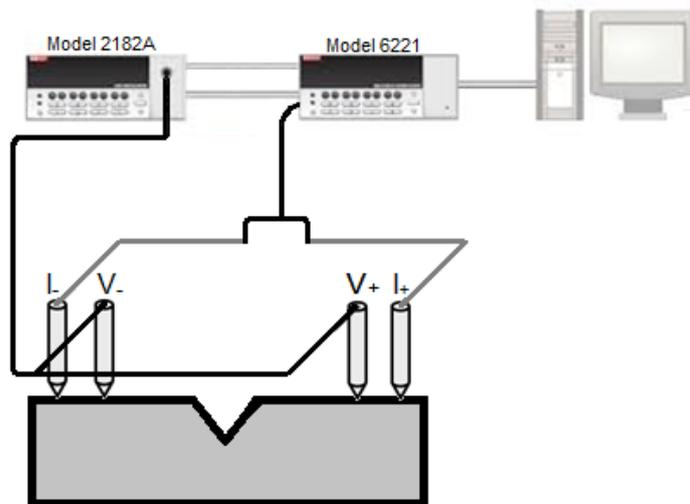
**Figure 1.** Measurement setup. The current feed into the specimen was through spring-loaded needle probes. The potential difference was measured using similar needle probes. The distance between two measurement points was 40.64 mm.
