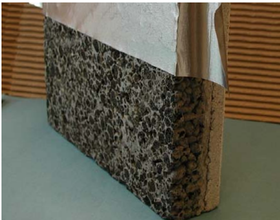
Light weight aggregate concrete with stucco
