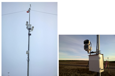
Figure 4. RSU installed in the visibility pole in Sodankylä Airport.
