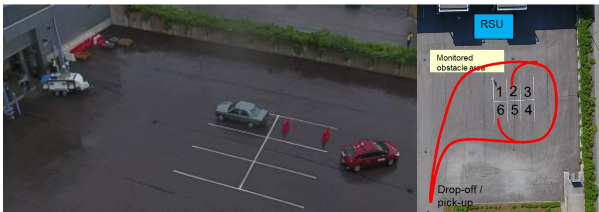
Fig. 3 - (a) Automated parking manoeuvre of the VTT parking place at Tekniikankatu, Tampere; (b) map of the area with the alternative routes to the parking spaces
