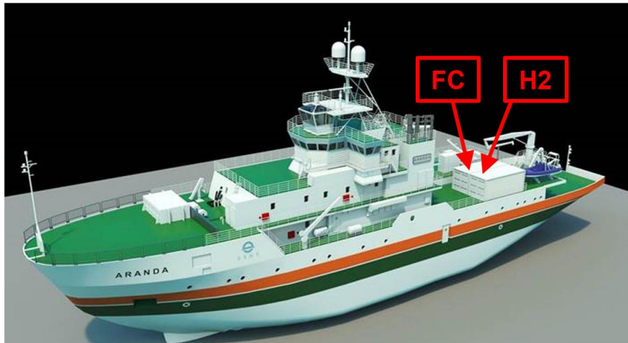
Fig. 3 - An illustration of the Aranda vessel and the FC and H2 containers' site on its deck. (N.B., in this illustration both containers are generic 20-foot containers.)
