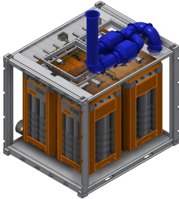
Fig. 2 - A CAD illustration of the H<sub>2</sub> storage container. Four gas cylinder bundles ("bottle packs") can be seen inside the container.
