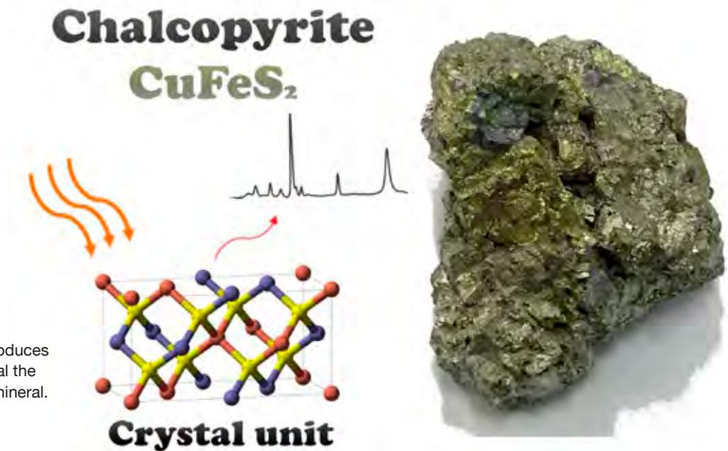
Figure 1. Laser excitation produces Raman photons, which reveal the fingerprint spectrum of the mineral.
