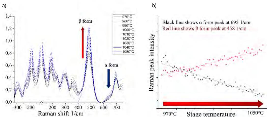
Figure 5. a) Spodumene phase transformation from the  $\alpha$ -form to the  $\beta$ -form during heat treatment can be observed from time-resolved Raman spectra, b) Raman peak intensity shows the rate of the transformation.
