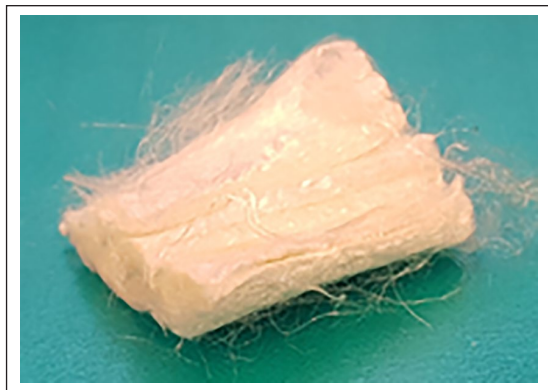
Figure 4. Viscose fibers of 24 mm length and 1.7 dtex linear density were used in the experiments.
