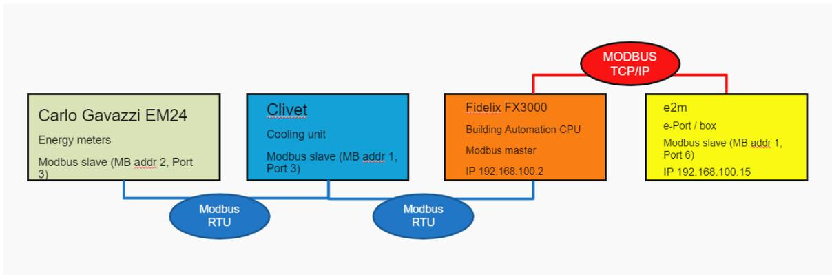
Figure 18. Connection for the Clivet Cooling Unit.
