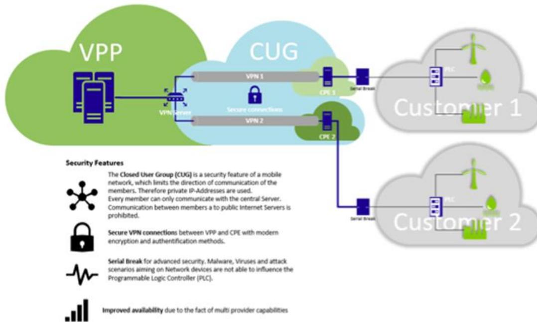
Figure 13. IT Security Concept of a commercial VPP (Source: e2m material)
