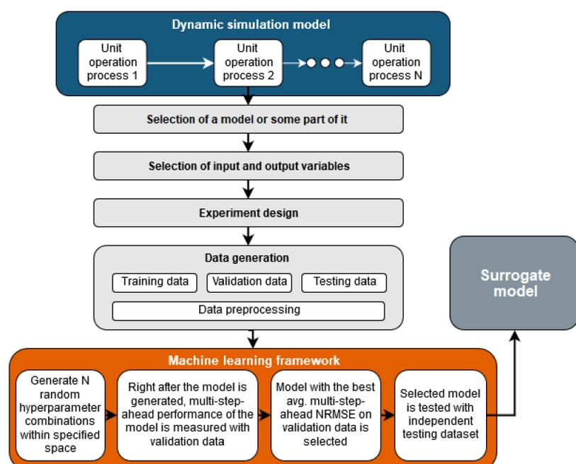
Figure 1. Overview of the surrogate modelling pipeline.
