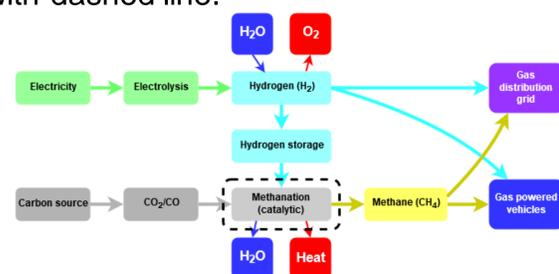
Figure 2. Process diagram of a power-to-gas process, showing how methane is produced using H<sub>2</sub> and CO<sub>2</sub>/CO (adapted from [2]).
