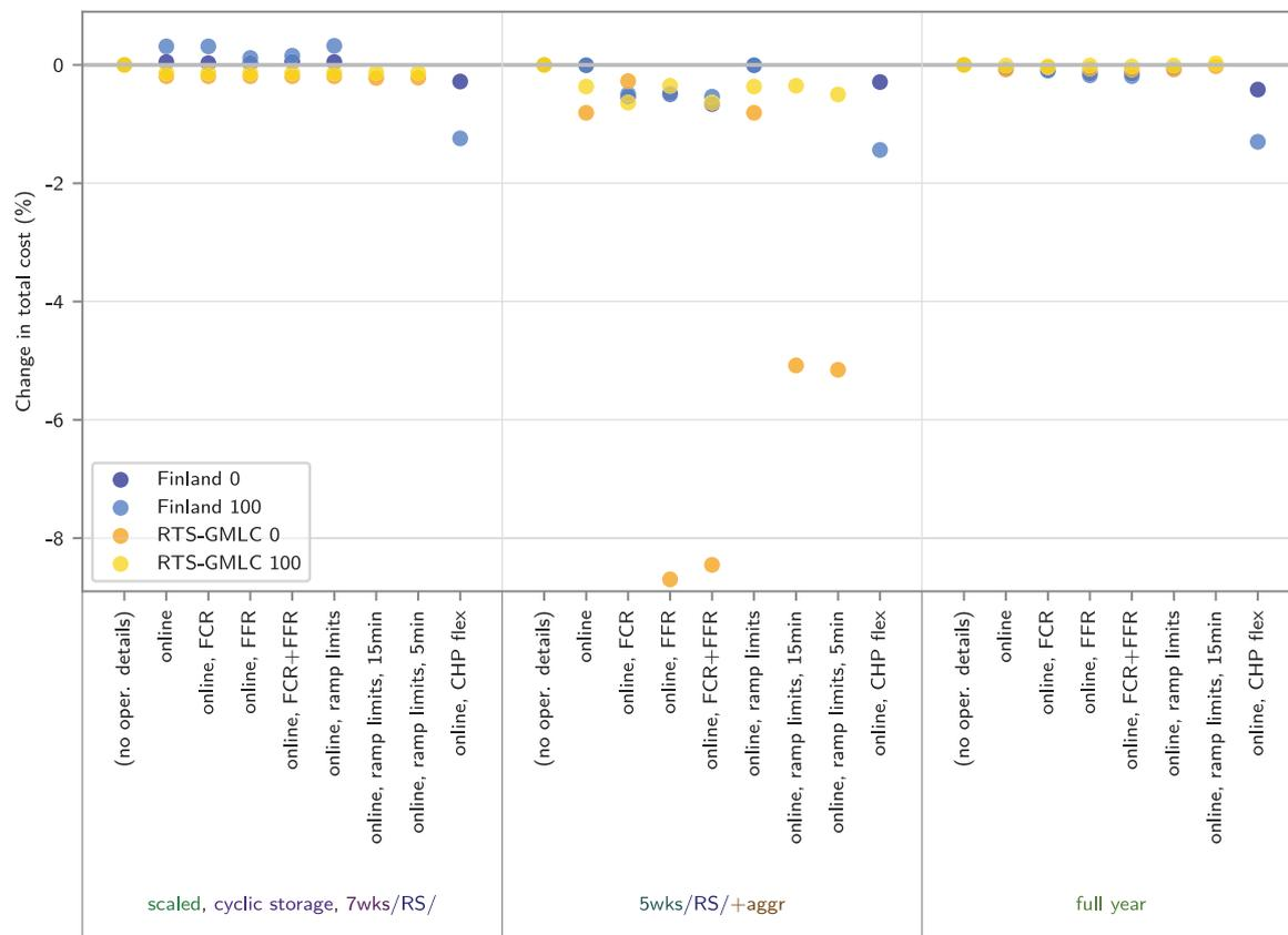
Fig. 5. Impact of operational details on annual system costs. All cases are compared to the corresponding ‘no oper. details’ case. CO<sub>2</sub> price €0 per tonne or €100 per tonne.
