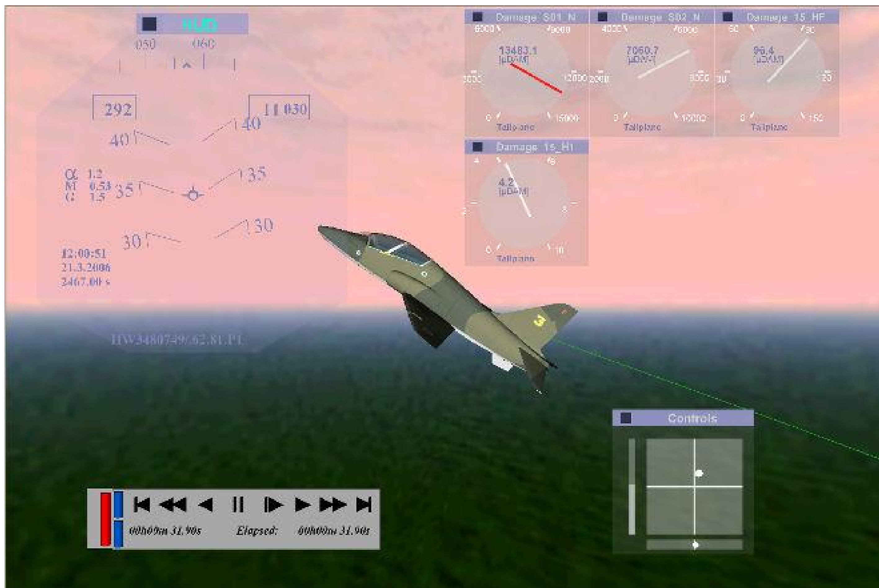
Figure 14: A snapshot from the visualization from the zoomed event of interest from Figure 13. Upper right: The analyst can follow the real time damage accumulation of several structural locations (4 locations shown) as the flight progresses. Upper left: Associated flight parameters are shown via the HUD (head-up display), which can be tailored as per the analysis needs. Lower right: Real time pilot controls (stick and pedals movements, throttle position) provide the analyst information on what the pilot was doing. Picture by courtesy of VTT.
