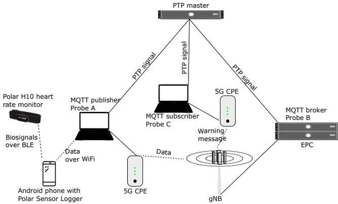
Fig. 3. Laboratory setup for the reliability measurements.
