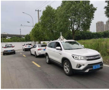
Figure 5. The OBU is placed on the top of the test car. The height of the antenna is about 1.5 m.
