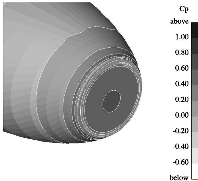
Figure 9. Pressure distribution on a pod with a small blunt aft end.
