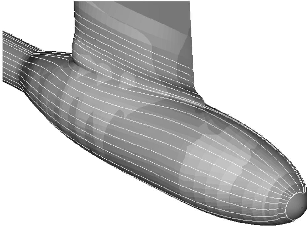
*Figure 10. Streamlines on the aft end of the final pod.*
