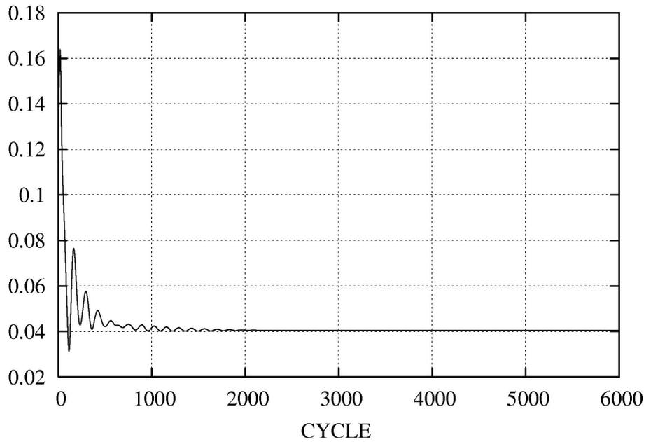
Figure 2. Example of convergence history for overall drag of a coarse grid.
