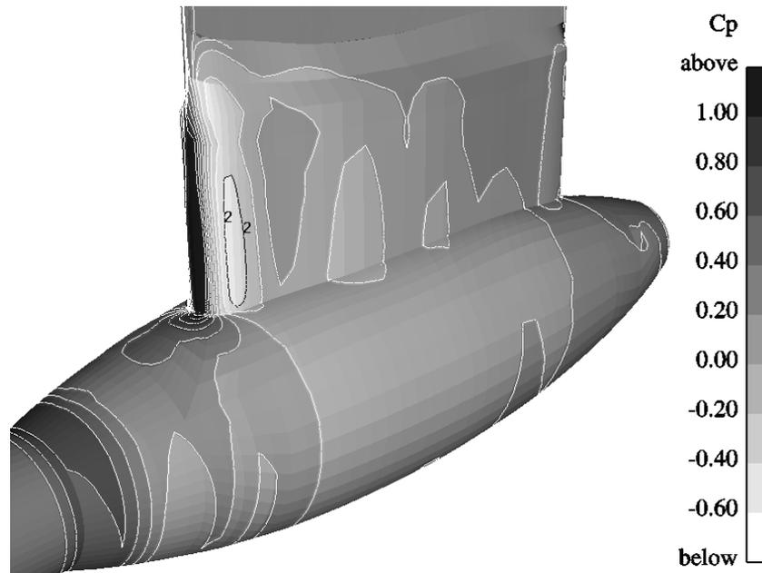
Figure 4. Pressure distribution on the initial version of the housing. Strut pressure side. The white color surrounded by contour labeled 2 shows pressure below the cavitation number.
