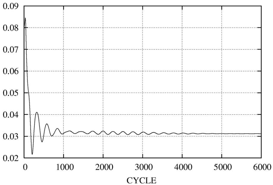
Figure 3. Example of convergence history for overall drag of a fine grid.
