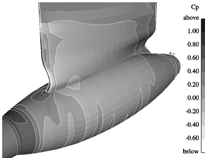
Figure 5. Pressure distribution on the asymmetric housing. Strut pressure side. The pressure falls no more within the lowest level in the scale.
