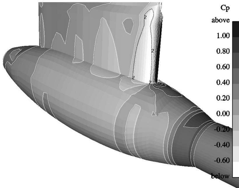
Figure 6. Pressure distribution on the initial version of the housing. Strut suction side. The white color surrounded by contour labeled 2 shows pressure below the cavitation number.
