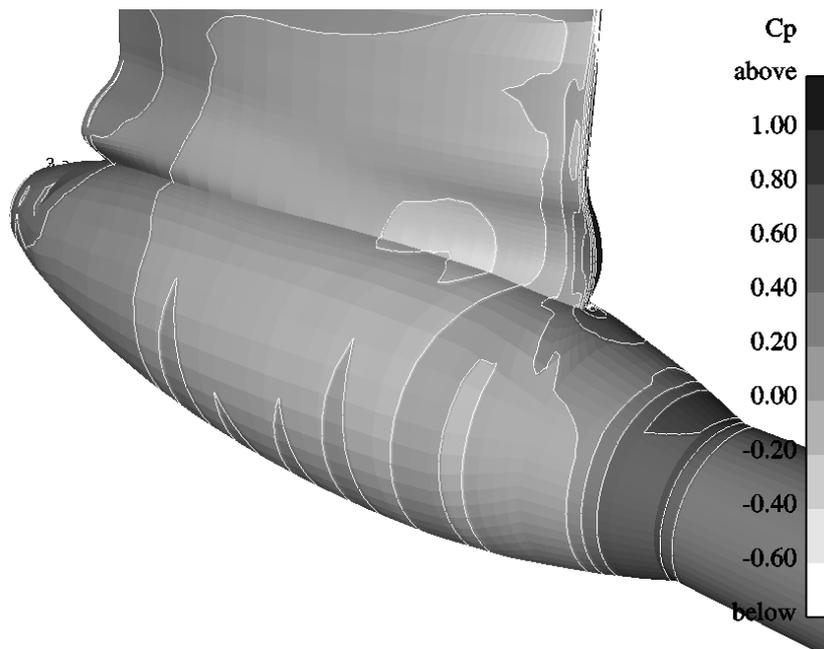
Figure 7. Pressure distribution on the asymmetric housing. Strut suction side. The pressure falls no more within the lowest level in the scale.
