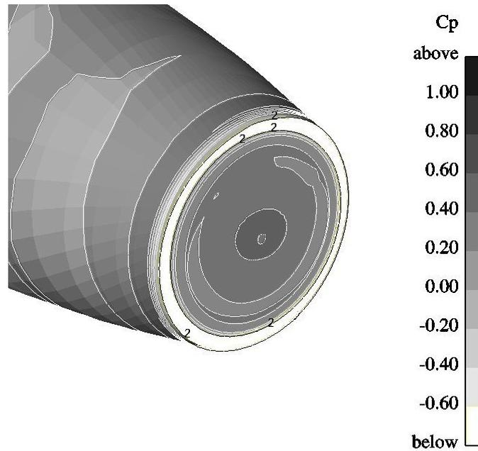
Figure 8. Pressure distribution on a pod with a large blunt aft end (initial shape). The white color surrounded by contour labeled 2 shows pressure below the cavitation number.
