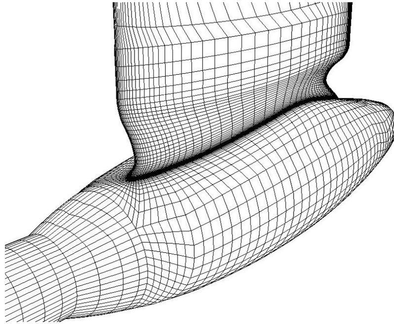
*Figure 1. Illustration of a coarse grid used for the first stages of the design. The strut is asymmetric. High resolution was confined to the portion of the strut located in the propeller wake.*
