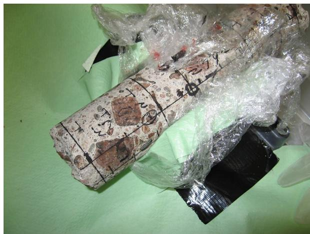
**Fig. 1** Picture of the FiR1 biological shield concrete core (diameter 7 cm)
