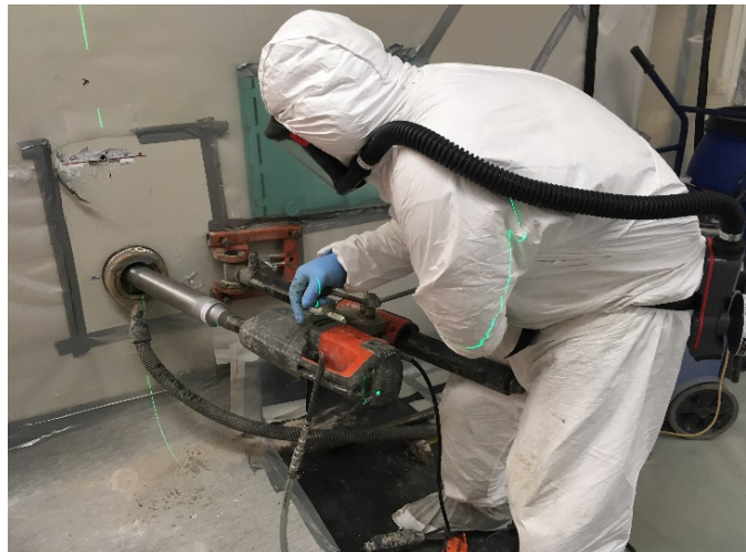
Figure 4: Left: Drilling directions towards the activated parts of the FiR 1 biological shield concrete (red lines 1, 2 and 3). Right: Drilling the specimens from the biological shield.
