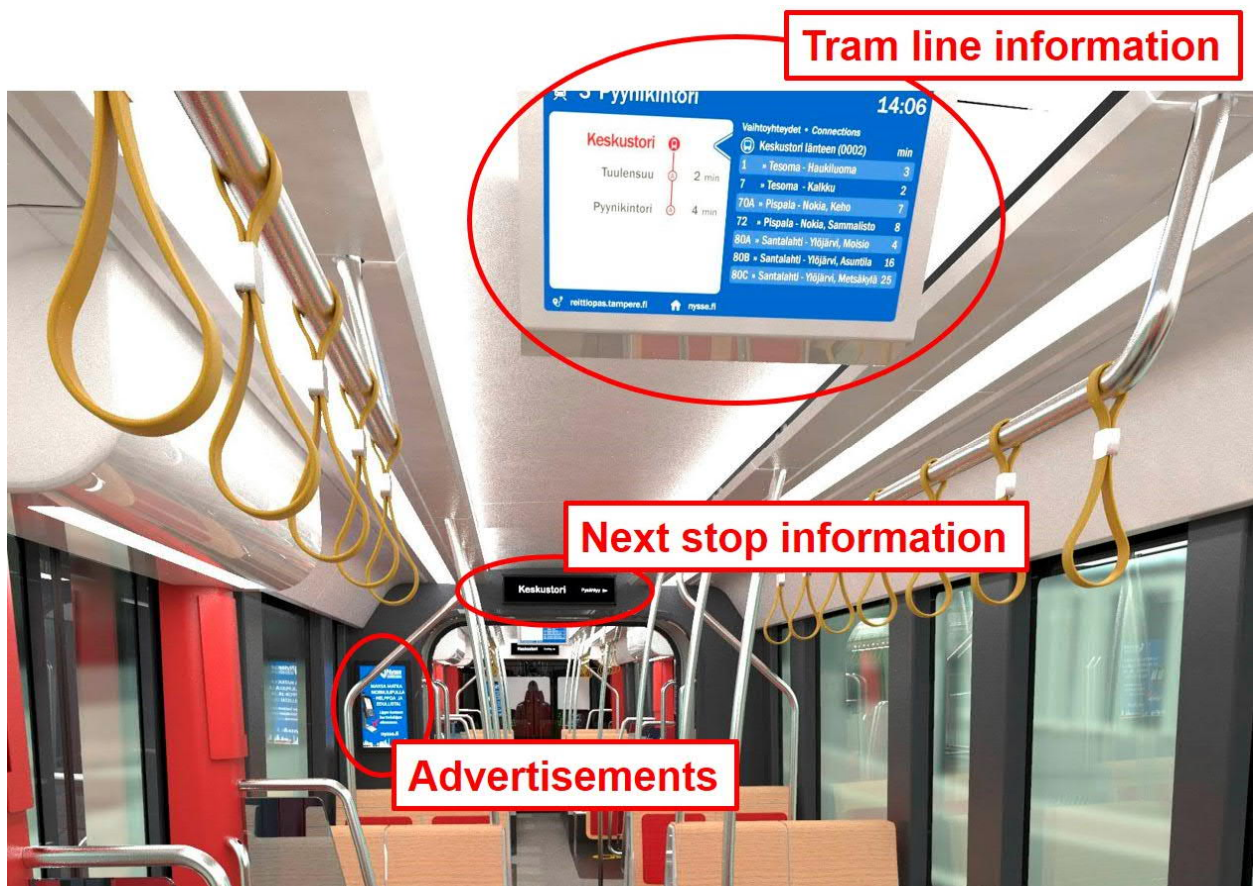
Figure 10. Displays and their purposes in the tram (Photo: Tampereen Raitiotie Oy).
