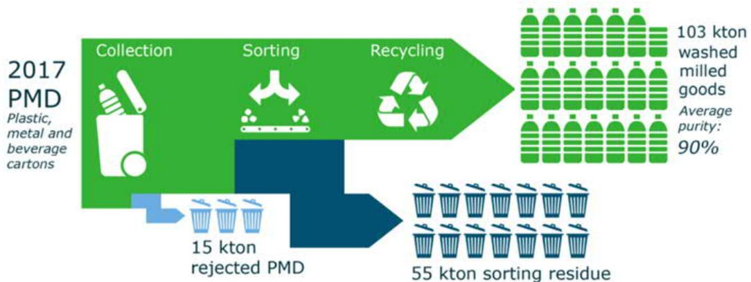
**Figure 4. Collection and recycling of post-consumer plastic waste. PMD = plastic, metal and beverage cartons. Adapted from Brouwer et al. (2019).**
