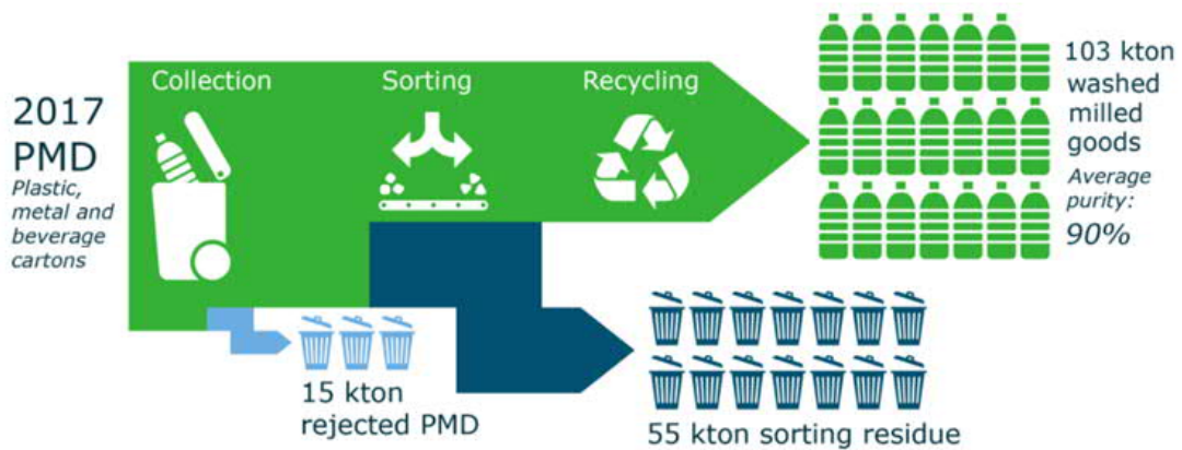
Figure 4. Collection and recycling of post-consumer plastic waste. PMD = plastic, metal and beverage cartons. Adapted from Brouwer et al. (2019).
